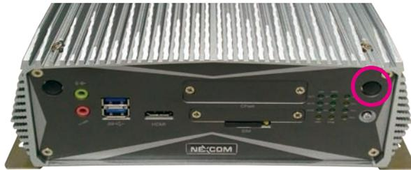
2. Install the antenna jack through the hole, and fix the cable with rings.
