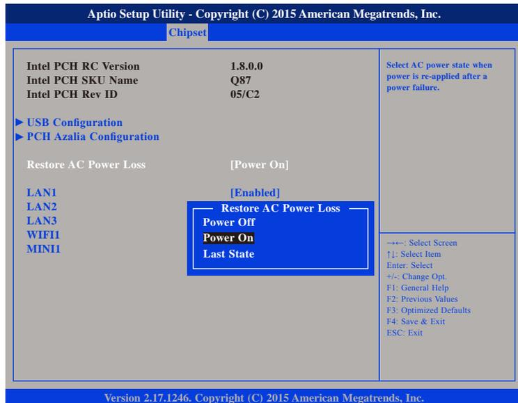
Selects the AC power state when power is re-applied after a power failure.
