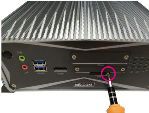
3. Secure the SIM card holder back to its original position.
