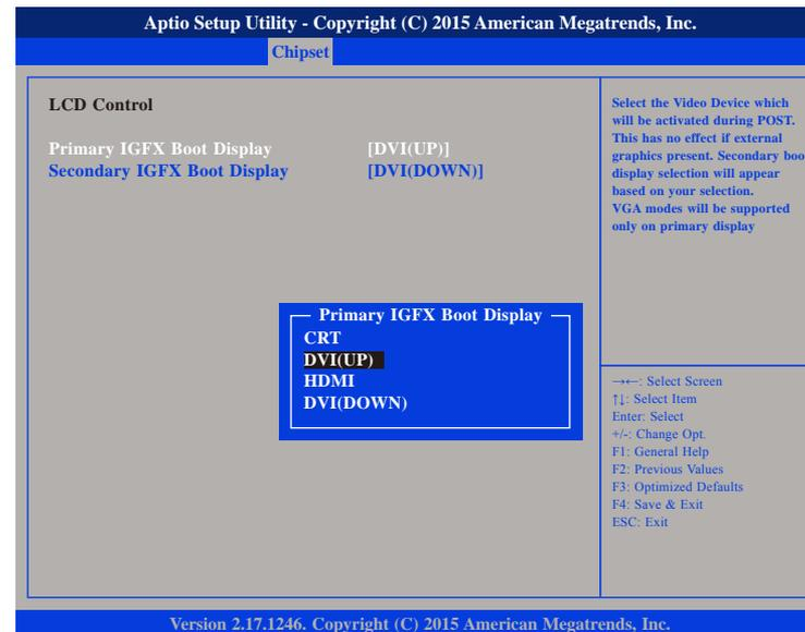
Selects the video device which will be activated during POST. This has no effect if external graphics is present. Secondary boot display selection will appear based on your selection. VGA modes will be supported only on primary display.
