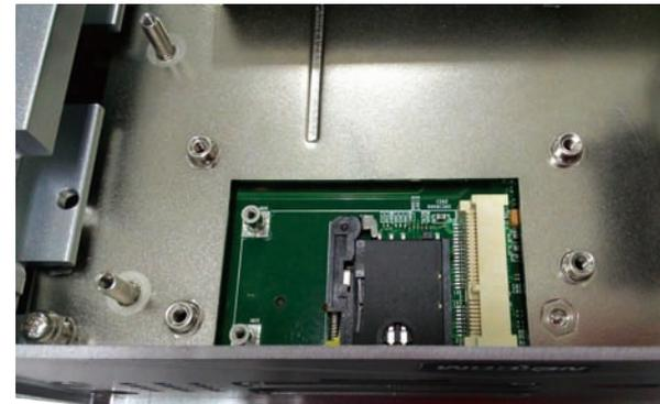
4. Insert the 3G module into the 3G/GSM slot and fix the cable onto the 3G module.
