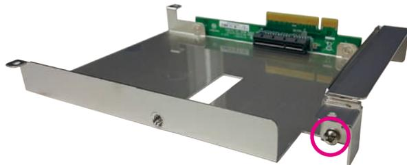
4. Insert the PCIe/PCI expansion card and fasten the screw to secure the card in place.
