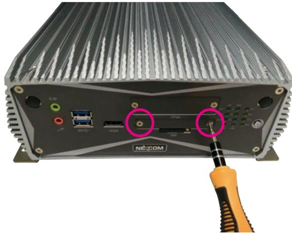
2. Insert the CFast card into the slot, then secure the cover back to its original location.
