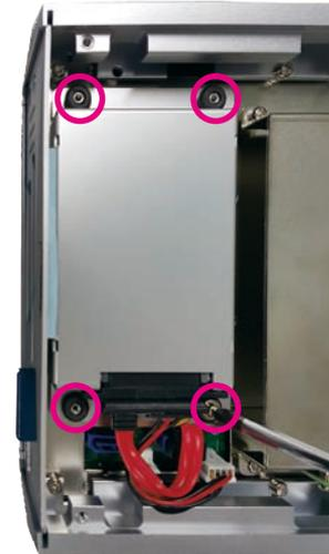
4. Place the HDD into the HDD bracket and secure the HDD with screws.
