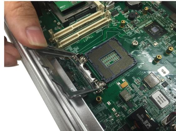
5. Insert the CPU into the socket. The triangular edge on the CPU must align with the corner of the CPU socket, while the two notches on the CPU must align with the alignment keys on the socket.
