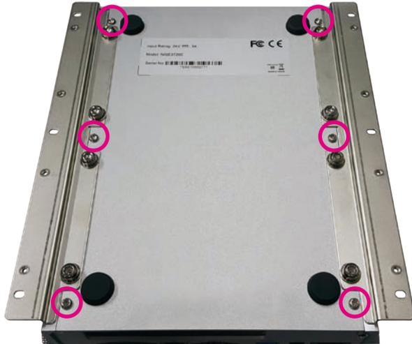
2. Remove the screws then lift up the bottom cover and remove it from the chassis.
