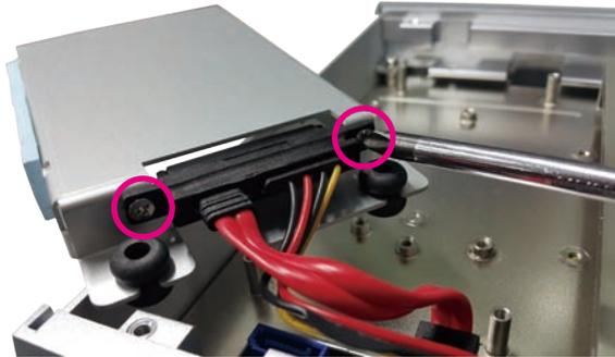
5. Connect the SATA connector to the HDD and secure the HDD bracket back to its original location.
