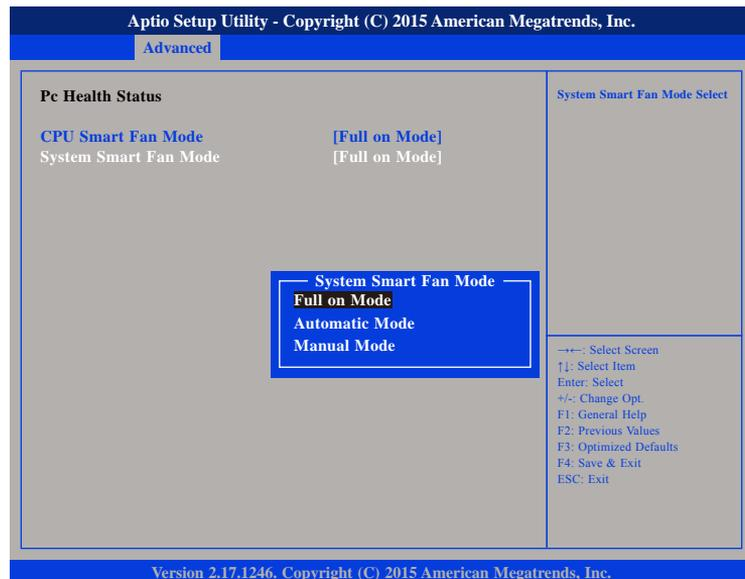
Configures the smart fan mode of the system fan, the options are Full on Mode, Automatic Mode and Disable Mode.
