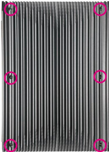
2. Remove the screws then lift up the cover and remove it from the chassis.
