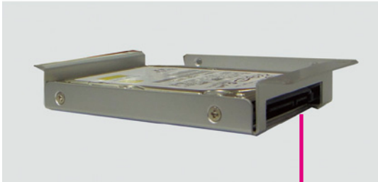
Connector side of the SATA drive
