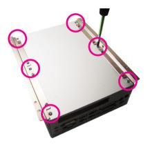
2. Remove the 4 mounting screws that secure the drive bay to the chassis then remove the drive bay. The drive bay is used to hold a SATA hard drive.
