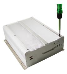
3. Lift up the cover then remove it from the chassis.
