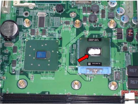
**Step 2.4: Insert heat sink silicon compound with screw**
