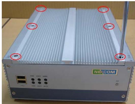
**Step 4: Secure the top cover with screws**
