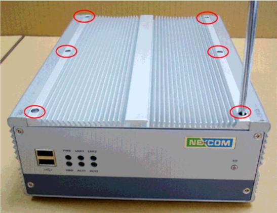
**Step 1: Remove 6 screws from the top.**
