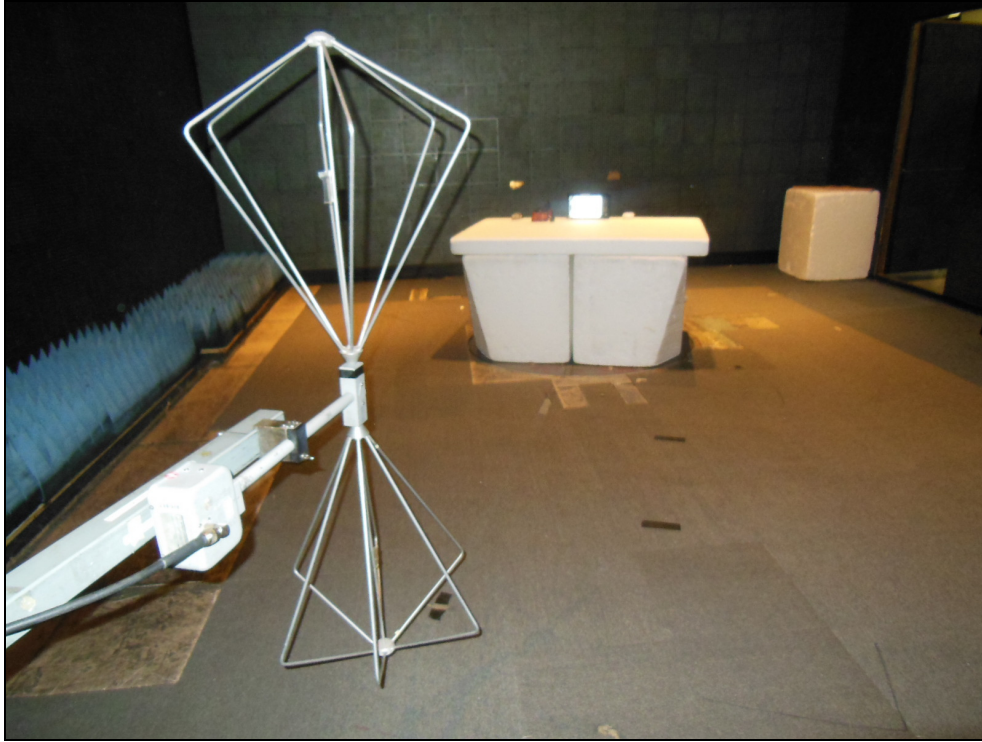
Figure 4.1.4-1: Radiated Emissions - Front View - SAC
