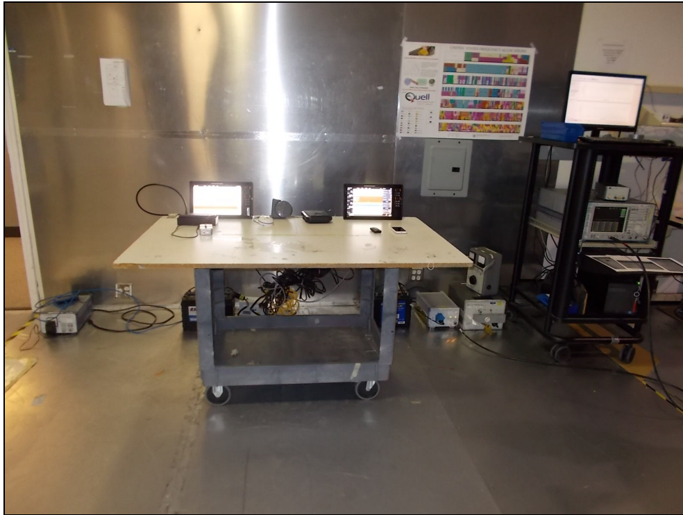
Figure 4.2.4-1: Conducted Emissions Test Setup – Front View
