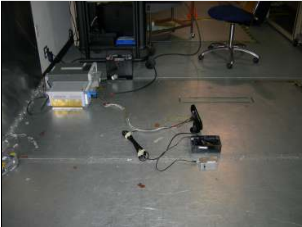
Figure 4.2.4-2: Conducted Emissions Test Setup – Side View
