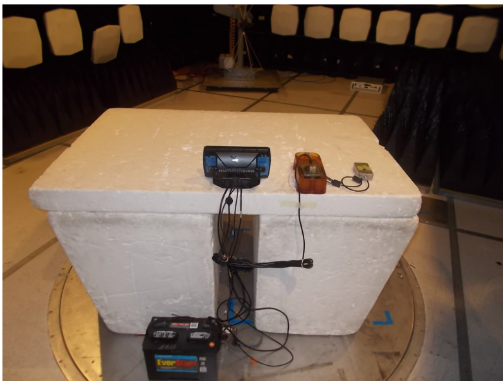
Figure 4.1.5-2: Radiated Emissions - Rear View
