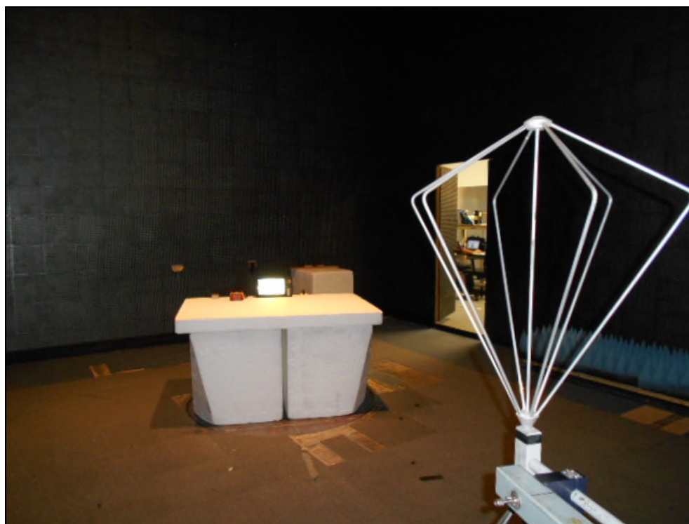
Figure 4.1.4-1: Radiated Emissions - Front View
