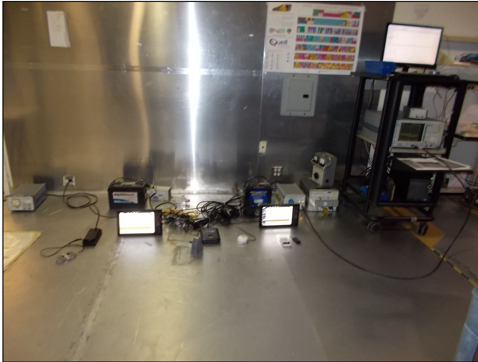
Figure 4.2.4-1: Conducted Emissions Test Setup – Front View
