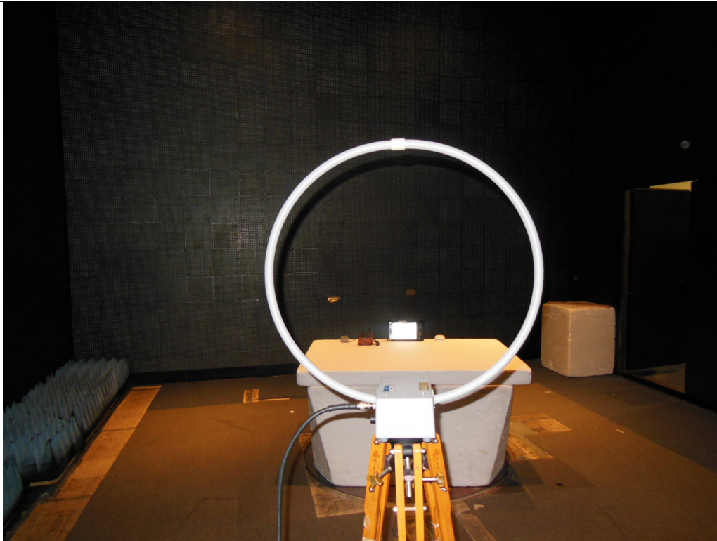
Figure 4.1.4-5: Radiated Emissions - Rear View - SAC
