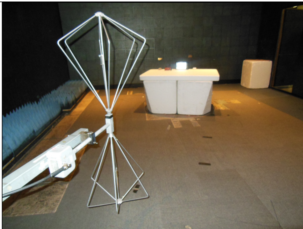
Figure 4.1.4-3: Radiated Emissions - Front View - SAC
