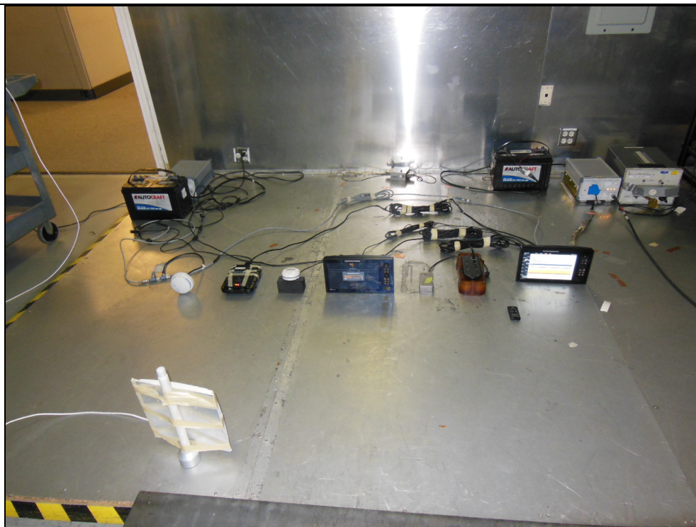
Figure 4.2.4-3: Conducted Emissions Test Setup – Front View - 60945
