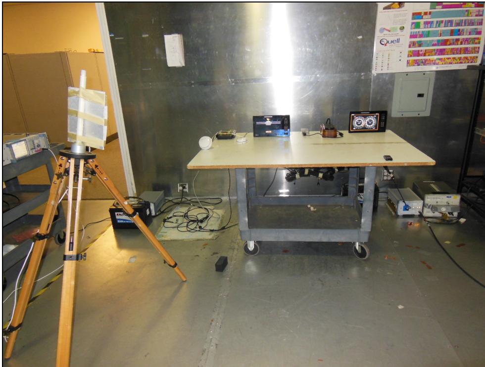
Figure 4.2.4-1: Conducted Emissions Test Setup – Front View
