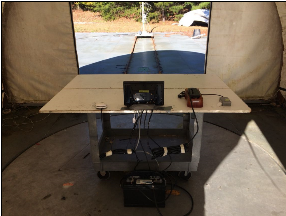
Figure 4.1.4-2: Radiated Emissions - Rear View - OATS
