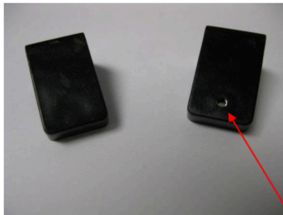
Original magnet holder on left. Current magnet holder on right. Notice that you can see the magnet through the pass-thru hole.
