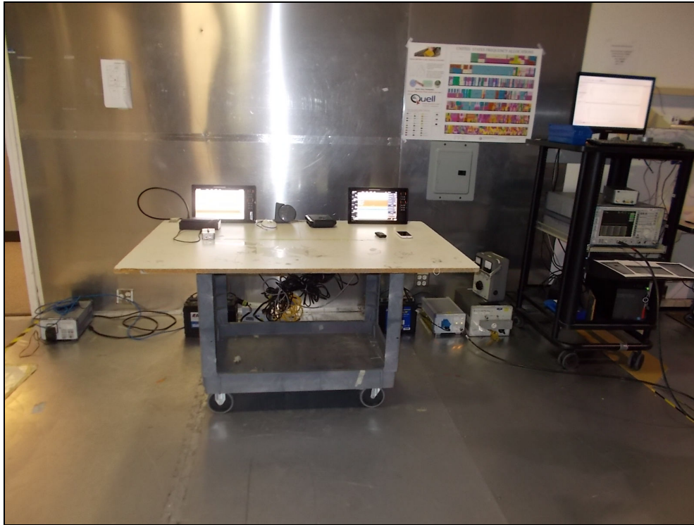
Figure 4.2.4-1: Conducted Emissions Test Setup – Front View
