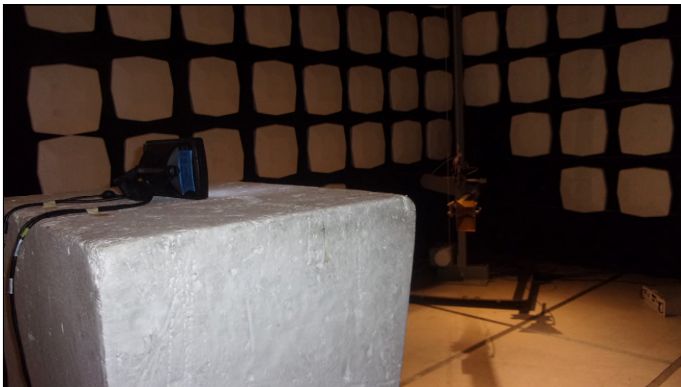
Figure 9-4: Radiated Emissions Test Setup
