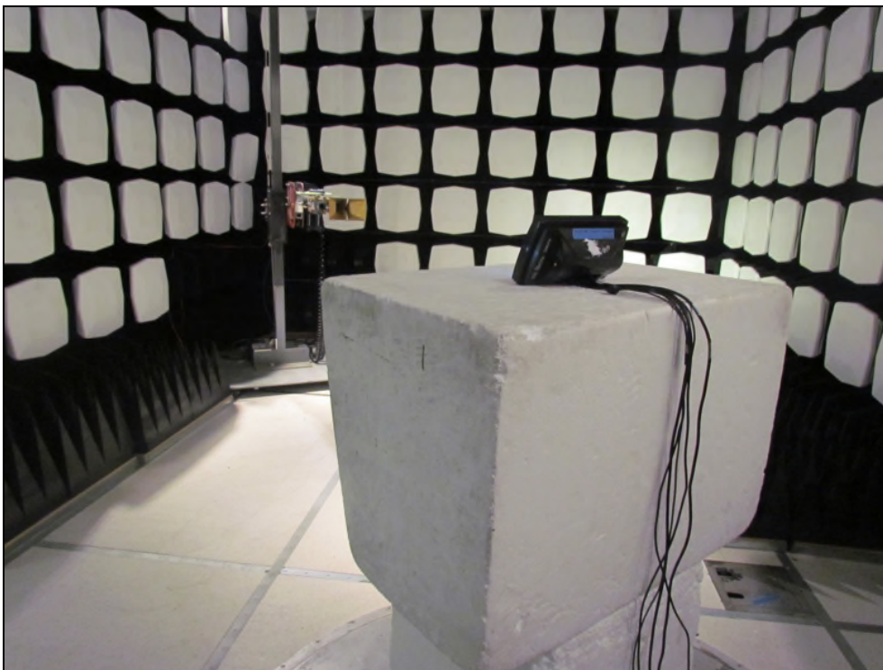
Figure 9-2: Radiated Emissions Test Setup
