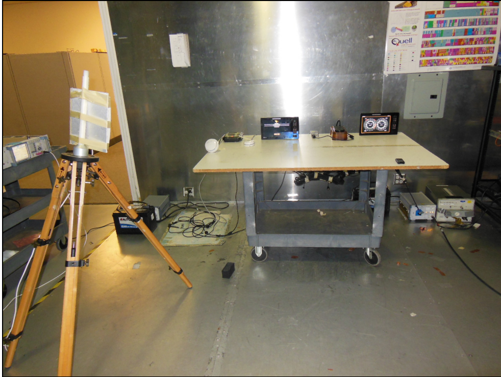
Figure 4.2.4-1: Conducted Emissions Test Setup – Front View
