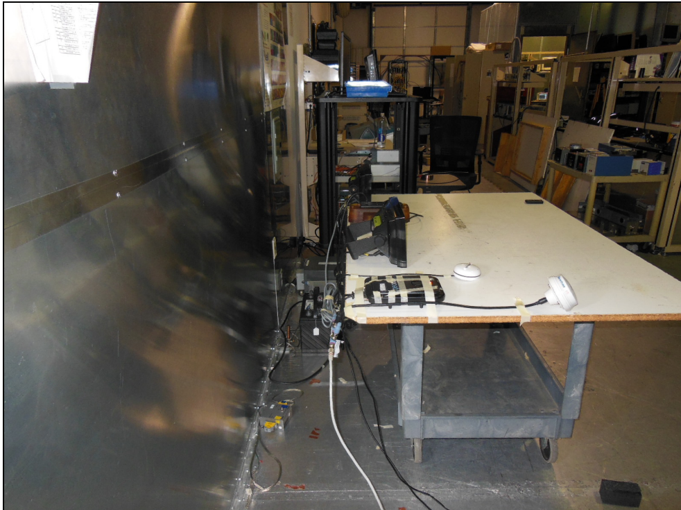
Figure 4.2.4-2: Conducted Emissions Test Setup – Side View
