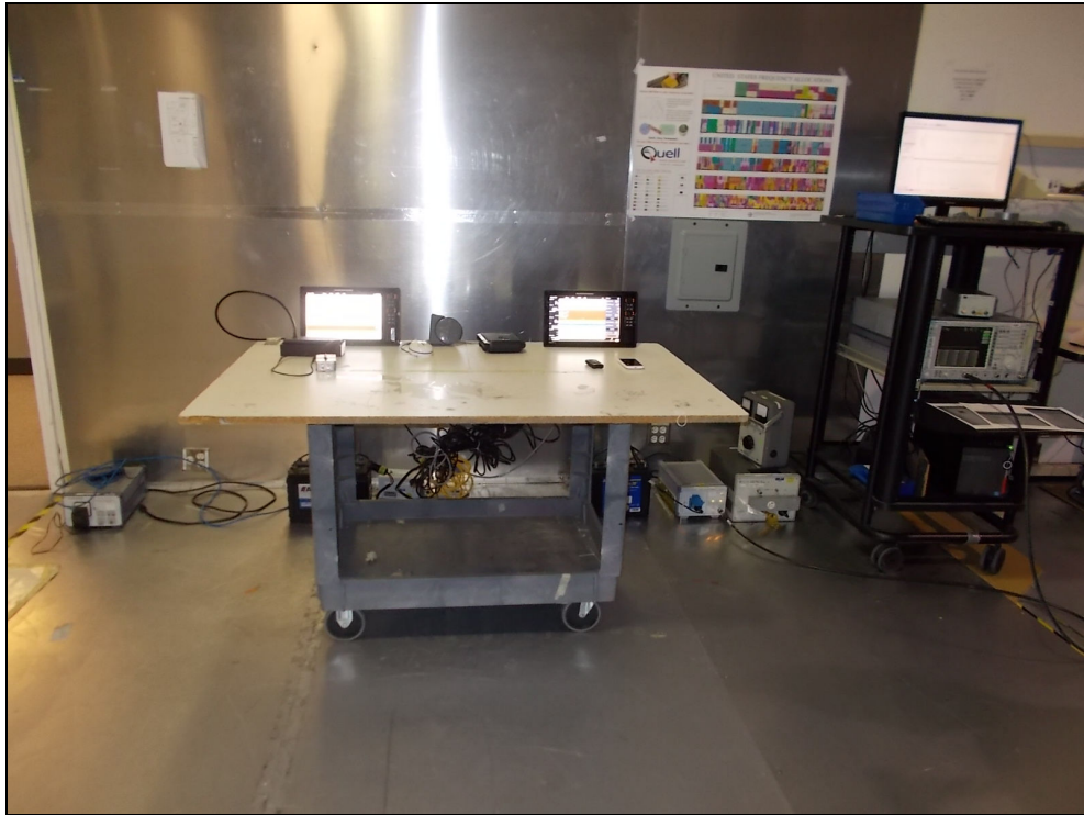
Figure 4.2.4-1: Conducted Emissions Test Setup – Front View
