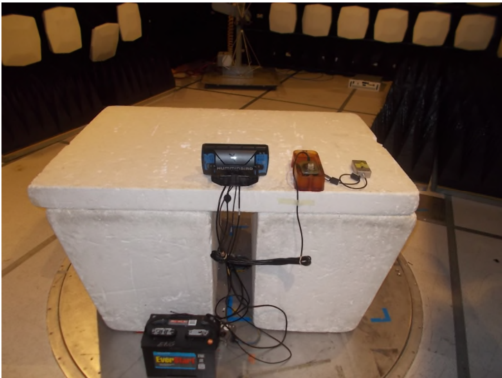
Figure 4.1.5-2: Radiated Emissions - Rear View
