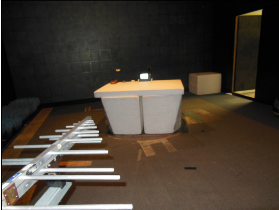
Figure 4.1.4-3: Radiated Emissions – Front View – Above 30MHz
