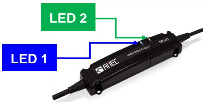
**NOTE:** LED 1 indicates receiving NMEA 2000 messages with blue flash light. LED 2 indicates receiving NMEA 0183 messages with green flash light.
