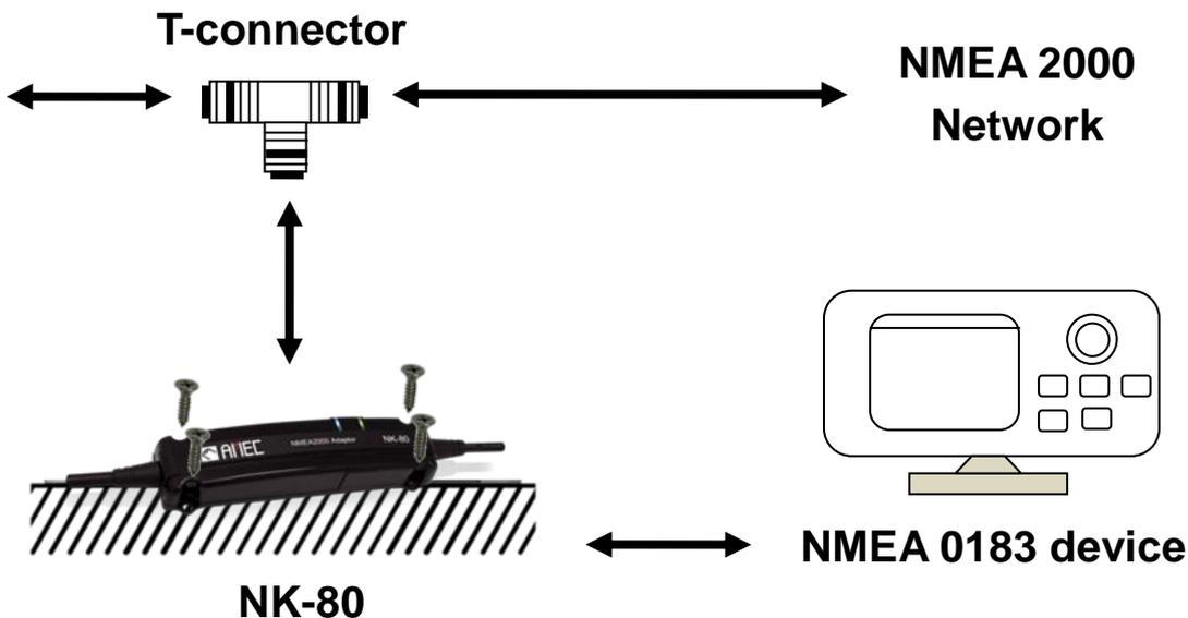
**Step 3:** Connect NK-80 Micro-C male port to T-connector Micro-C female port. If the provided cable length 0.1M is not enough, use an extension cable with proper length for connection.
