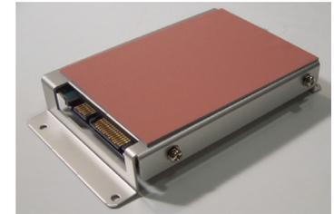
5. Connect the SATA data cable and SATA power cable to the connectors on the SATA drive.
