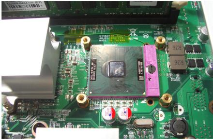
6. Before you install the heat sink, apply thermal paste onto the top of the CPU. Do not spread the paste all over the surface. When you later place the heat sink on top of the CPU, the compound will disperse evenly.
