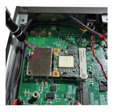
4. Push the module down and secure it with a screw.
