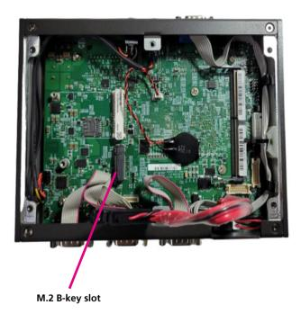
2. Make sure the gold-plated six-pin connector on the edge of the module is on the left, while the five-pin connector is on the right.
