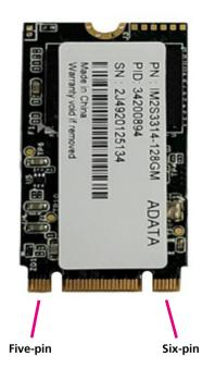
3. Insert the M.2 module into the M.2 slot at 45-degree angle until the gold-plated connector on the edge of the module completely disappears into the slot.
