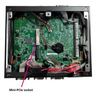
2. Install the mini-PCIe bracket to the mini-PCIe module. (When using a half-size module)
