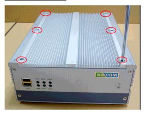
Step 1: Remove 6 screws from the top. <u>Install/Remove CPU</u>
