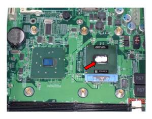
Step 2.4: Insert heat sink silicon compound with screw
