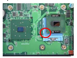
Step 2.2: Be aware that the beveled corner of the CPU as shown in the picture is aligned to the direction of the socket.
