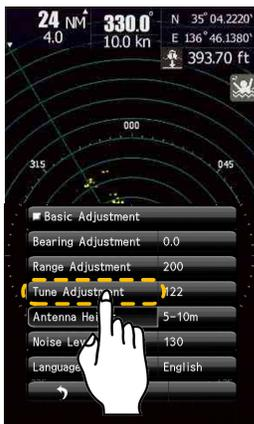
② Rotate the Rotary knob to set the tuning.
